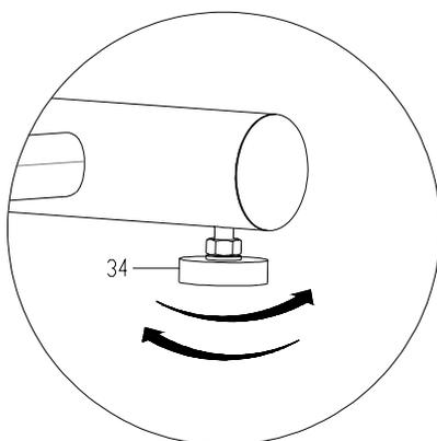
When this product is on an uneven surface, please adjust both Foot Pads (34) according to the above instruction picture.
